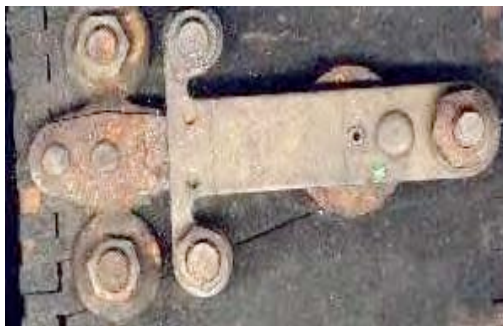
POINTS END OF SPARK COIL USED TO MAKE SENDING KEY
